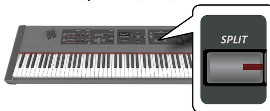
The Keyboard is divided into two sections. The region of the keyboard to the left of the split point becomes the Lower part , while the region of the keyboard to the right of the split point becomes the Main part.
