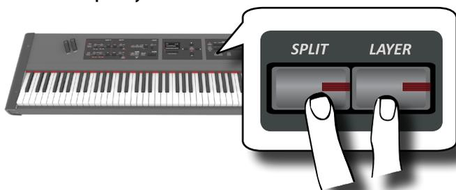
The Keyboard is divided into two sections. The region of the keyboard to the left of the split point becomes the Lower part while the region of the keyboard to the right of the split point becomes the Main and Coupled part.
