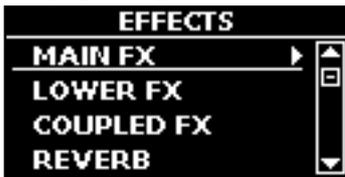
2. Use the [▲], [▼] and [▶] button to select one of FX page relative to the keyboard part ("MAIN FX", "LOWER FX" and "COUPLED FX").
