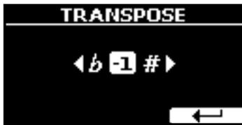
2. Use the [◀] [▶] buttons to adjust the transposition value.
