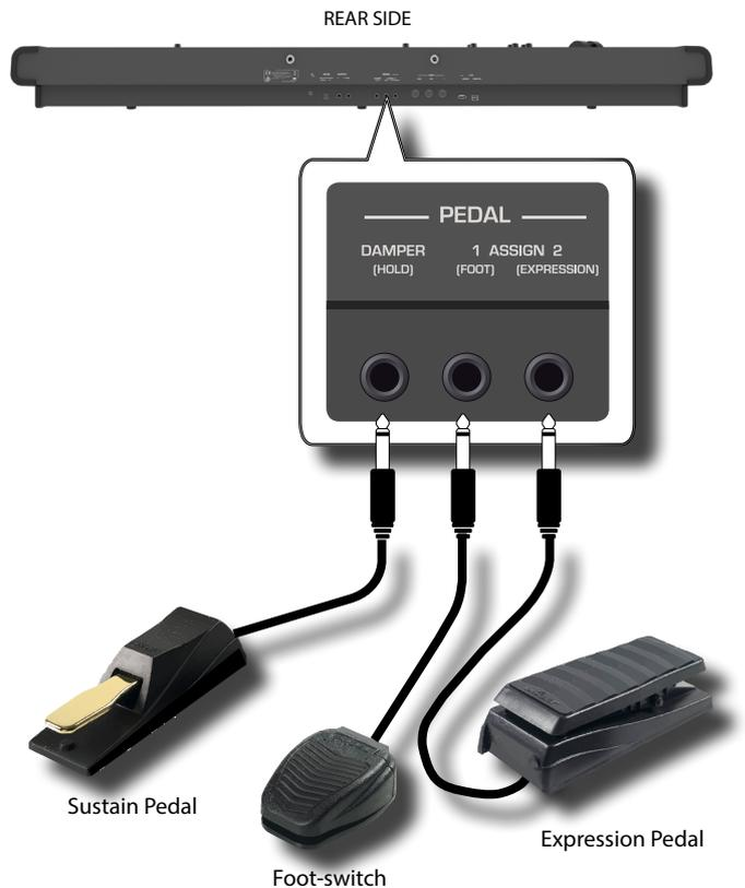
1. Connect to the DAMPER (HOLD) socket a sustain pedal. This is the most commonly used pedal in a digital piano. When pressed, all notes played will continue to sound until the vibration naturally ceases.
