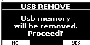
1. Press the "YES" Function button to safely remove the USB Memory.
